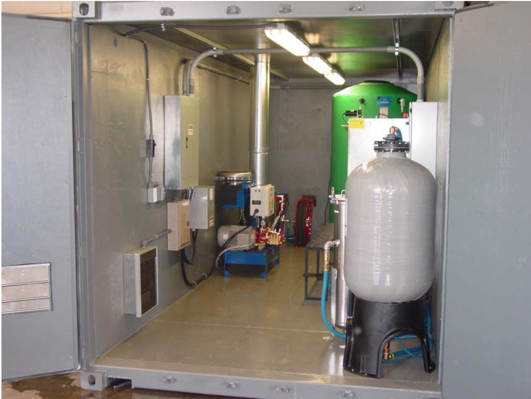
20' hardened enclosure with Cyclonator Deuce, hot water pressure washer, water cannon, two hose reels mounted at back, high pressure auto backwashing media filter in foreground NEMA 4 electrics, automatic energy saving lights
