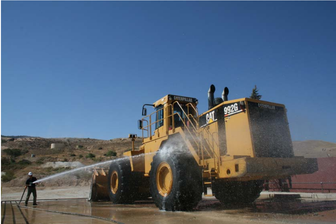
Riveer Environmental 100 PGM @100 PSI water cannon
